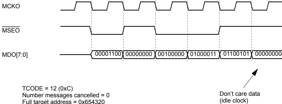
Figure 24-41. Indirect Branch Synchronization Message
